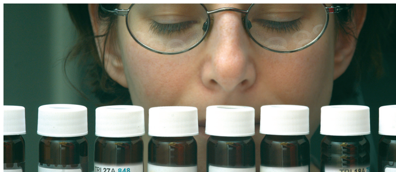
Figure 1. The tools of the psychophysical trade: an informed, consenting human subject and an odor source. Odorants are supplied by a variety of means: squeeze bottles, 'rip-and-sniff' packets, glass vials (as depicted here), or sophisticated computer-controlled olfactometers that deliver odors in a stream of warm and humidified air directly into the nose. Photo by Zach Veilleux, Rockefeller University Communications and Public Affairs.
